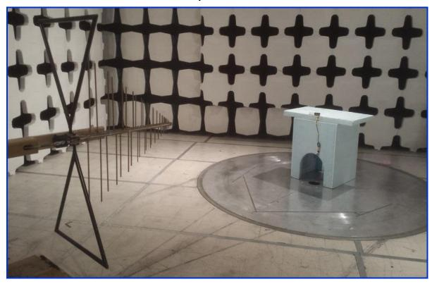
Photo of Radiated Emissions test setup: EUT Orientation
